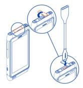
2 Connect an HDMI cable to the adapter, and then to the HDMI connector of a TV. You may need to manually select the HDMI input on the TV.
